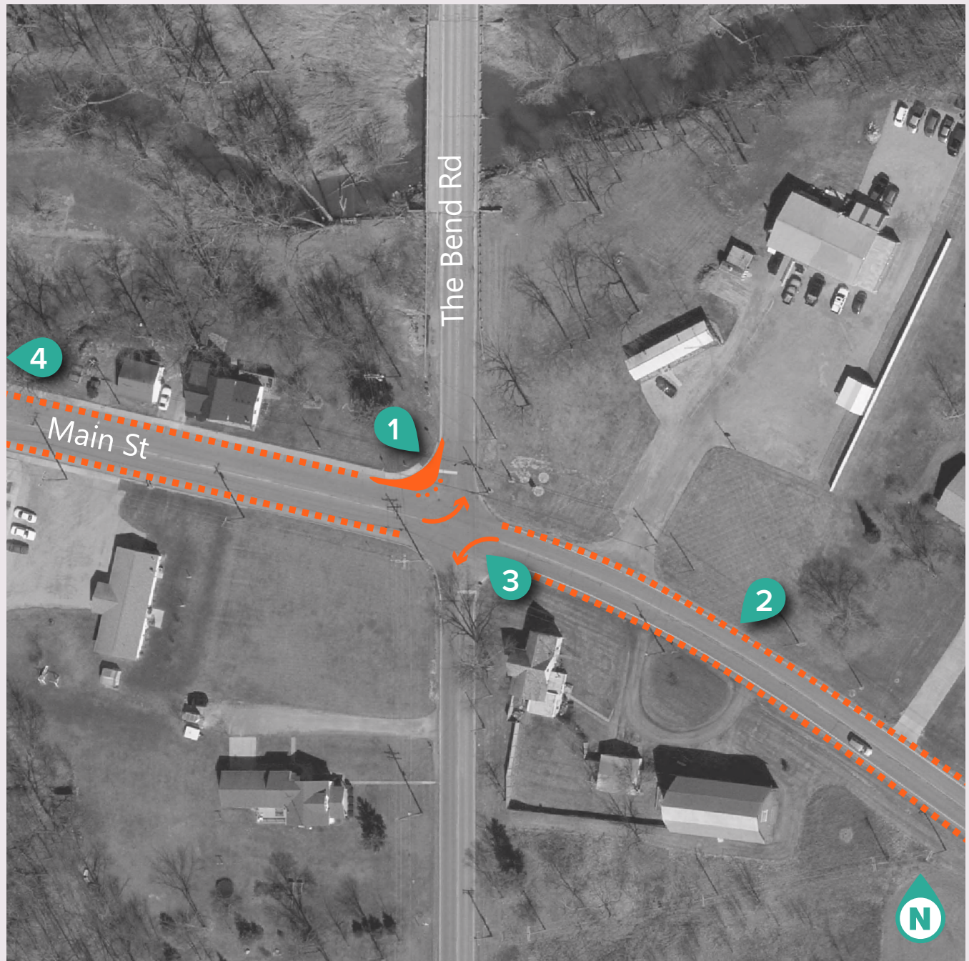
| Concept illustration of recommended safety improvements at SR 15 (Main St.) and The Bend Rd. in Defiance County
